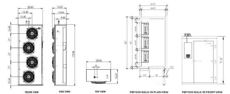
PBF1200-TS includes three evaporator coils
