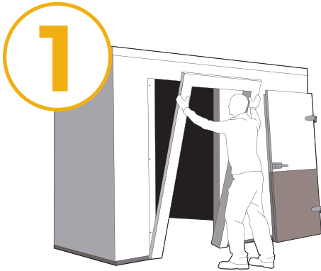
1 Set the replacement frame in place.
