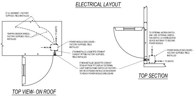
ALL WIRES STUBBED UP FROM INTERIOR OF ROOM FOR CONNECTION TO POWER MODULE MUST BE TAGGED AND LABELED FOR FIELD CONNECTION PER THE FOLLOWING CONVENTION (REFERENCE SMARTRITE 100 WIRING DIAGRAM SMRT100WD):
