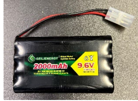
Battery (Factory installed in TFT enclosure)
